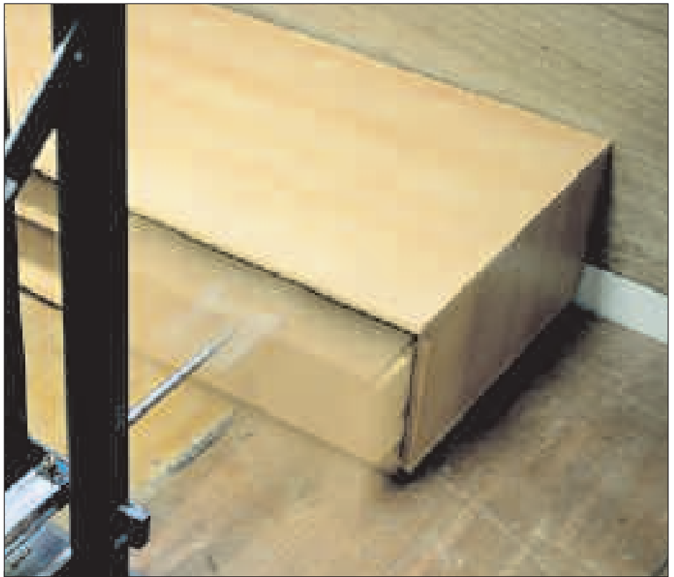
Drawer testing in SATRA's laboratories. Test methods in the relevant EN standards ensure that furniture meets expectations for safety and function.
